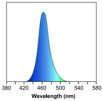
Fig.1. Emission spectrum for the BLooK LED transilluminator
