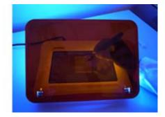
Note: For cutting fluorescent samples out of the gel, please lift the lid to access the gel.
